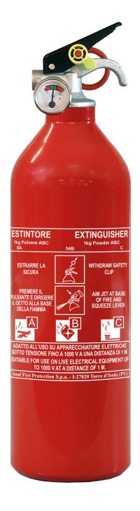
PS1-XM TOP is a stored pressure, multi-purpose dry powder fire extinguisher with pressure gauge. Wide operating temperature range –30°C + 60°C, ensures suitability for use in low-temperature countries. Certified to the Pressure Equipment Directive PED 2014/68/EU, to the Marine Equipment Directive MED 2014/90/EU and EN3-7. 100% of the fire extinguishers are checked by an electronic helium leak detection system.
